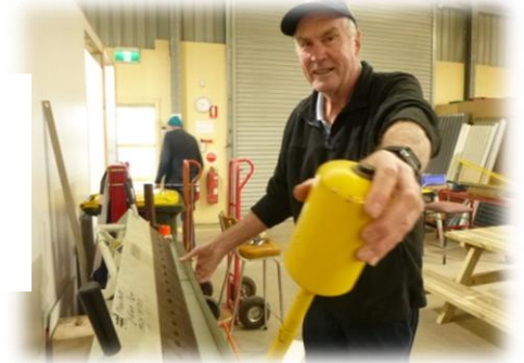
Alan using the metal folder to make corner angles for raised garden beds
